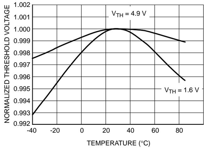
Figure 8. Normalized Reset Threshold Voltage vs. Temperature
