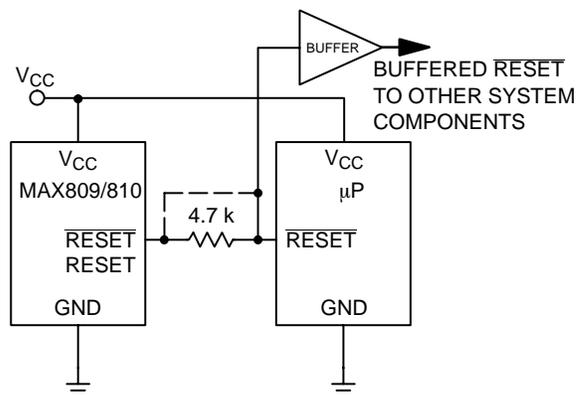
**Figure 4. Interfacing to Bidirectional Reset I/O**
