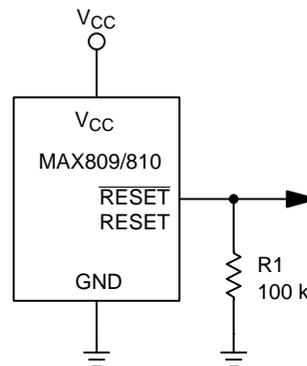
**Figure 3. Ensuring RESET Valid to V<sub>CC</sub> = 0 V**
